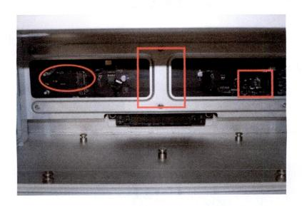
Step 2b: Please note, due to small size and delicate nature of the parts, this step should be done very carefully. If you acquired the Bluetooth antenna, please connect it to the Bluetooth connector on the card. Since the environment can be different, there is no perfect place for the antenna. The antenna is best to be placed closest to your keyboard and mouse.
