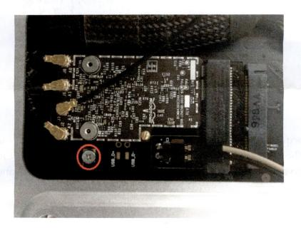
**Step 2:** Carefully attach RP-SMA cables to U.FL connectors as shown below. (Given that Mac Pro have only three antennas and BCM94360CD and BCM94331CD requires four, you will need an additional antenna or extension cable).
