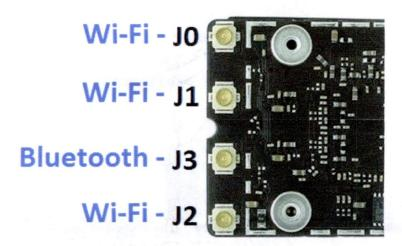
**Step 2a:** If you acquired the Bluetooth antenna extension, please connect the female side of this extension to the Bluetooth connector on the card. The opposite end of the antenna extension has to go behind the central column (custom USB cable as well) and connect with the original Bluetooth antenna cable (disconnected from the old original Bluetooth card).
