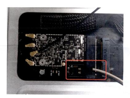
**Step 5:** The opposite side of the custom USB cable connects to the disconnected 4-wired cable from the old Bluetooth card.
